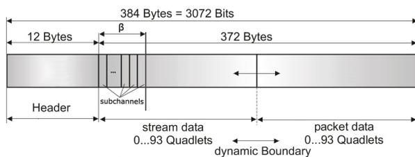
**Figure 3 – MOST frame with subchannels**
